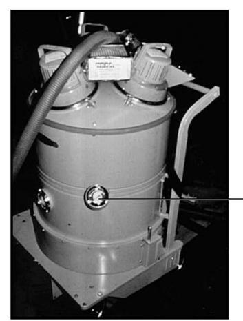
Figure 14.1b Pressure Gauge Indicator Shows When Filters Require Changing.
