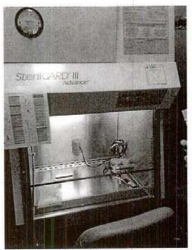
Photo 4: Type 2A biological safety cabinet, located at the west end of Building 6A.
