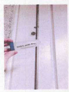
Photo 11: Paint chip sample 100814-WIFR-B-01 collected from the south concrete wall.
