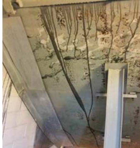
Photo D6. Lubricant dried to the back of the bullet trap panel.
