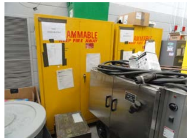
Flammable cabinets blocked by equipment
