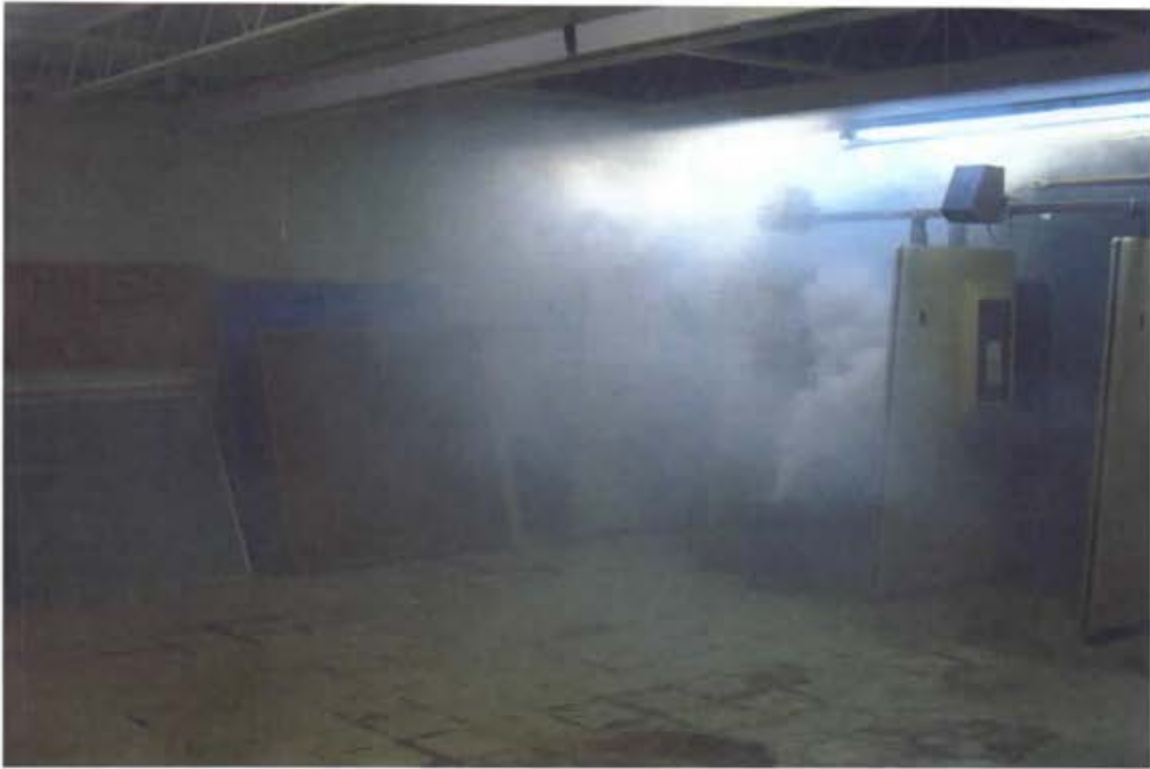
Photo 13: The smoke is being blown towards the observation deck as a result of air rushing through the dropped ceiling opening.
