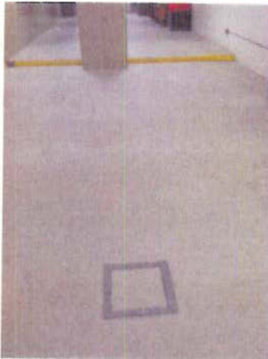
Photo 7: Lead wipe floor sample 10412-Lewistown-06 from the northern end of the converted Indoor Firing Range.
