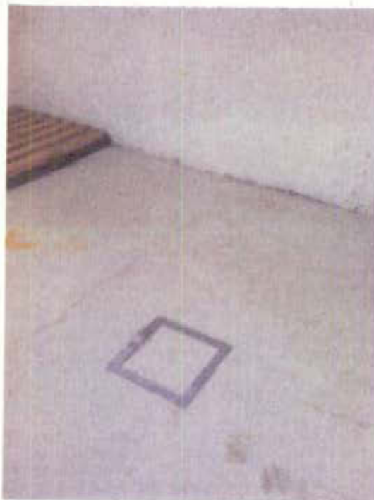
Photo 8: Lead wipe floor sample 10412-Lewistown-07 from the storage locker, south end of the converted Indoor Firing Range.
