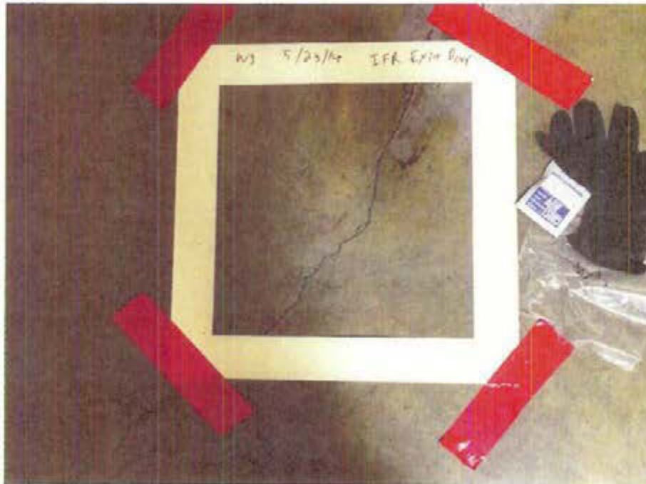
Photo 13: Lead Wipe Sample W3; Drill Hall Near IFR Exit Door.
