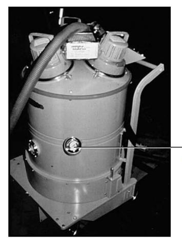
Figure 14.1b Pressure Gauge Indicator Shows When Filters Require Changing.
