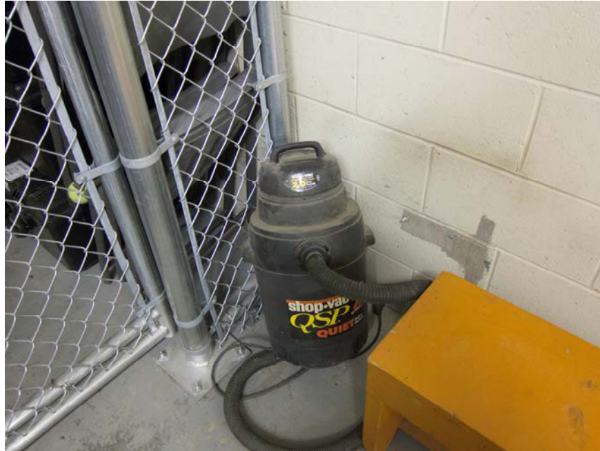
Shop vac inside the converted firing range note that only HEPA vacuums should be used in a lead dust hazard area
