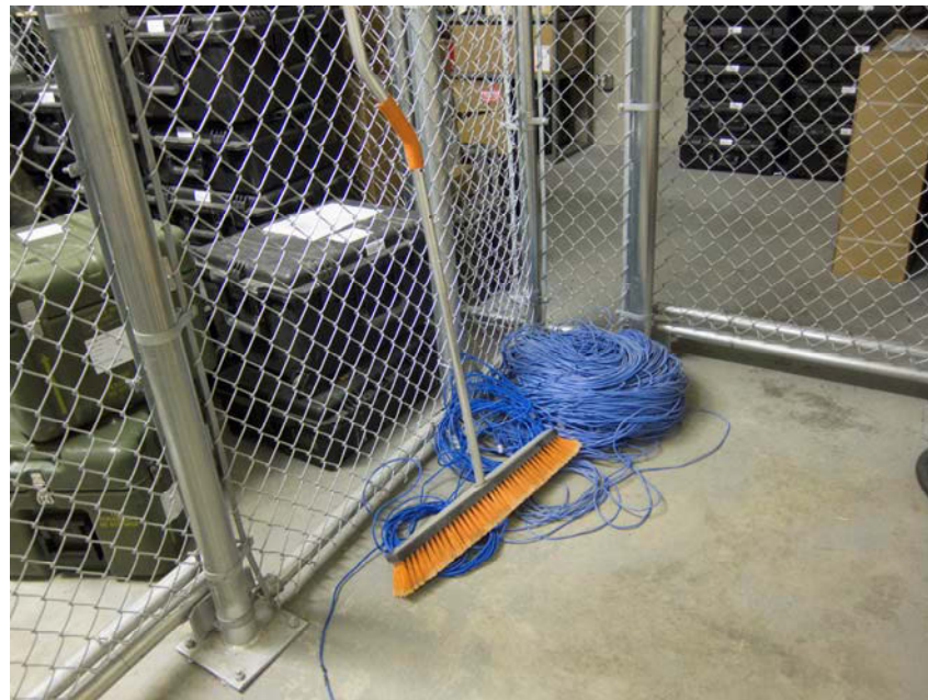
Broom inside the converted firing range, note that dry sweeping should not be performed in a lead dust hazard area
