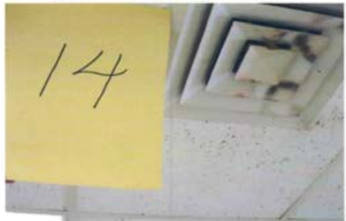
Lead wipe sample 14, located on the supply air grill in the orderly room
