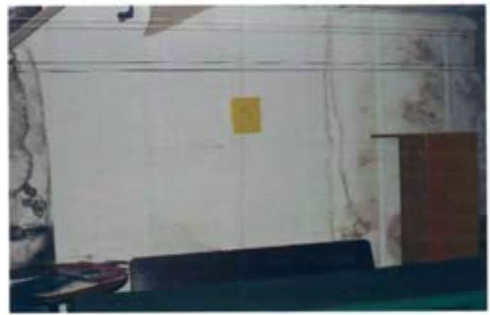
Lead wipe sample 5, located on the right acoustic tile wall of the range
