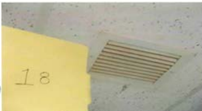
Lead wipe sample 18, located on the return air grill in the supply NCO office
