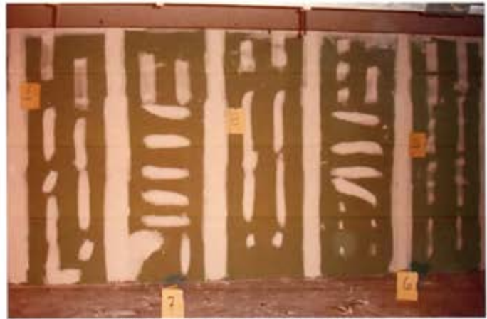
View of Lead wipe sample 1,2,3,6, and 7, located on the drywall of the former backstop area
