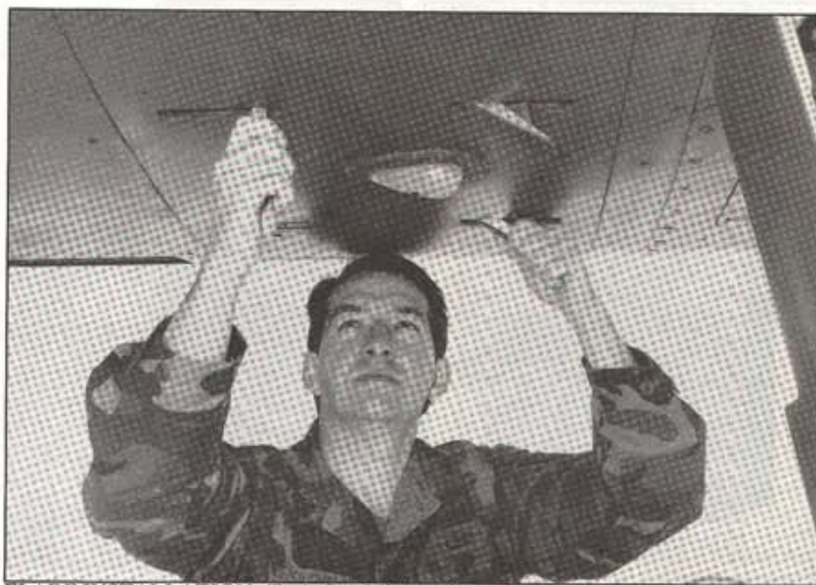
FLARE INSTALLATION - Tech. Sgt. Michael Duvall installs a flare canister in an A-10 Thunderbolt flare pod in the main landing gear. (Photo by Tech. Sgt. James Foard, Maryland National Guard).
