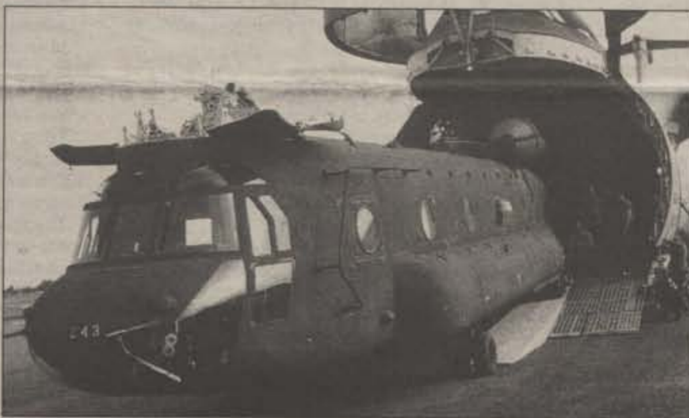
BRINGING RELIEF - Army Guard aviation mechanics (above) from Connecticut and Illinois use a crane hoist and guide straps to reassemble a CH-47 Chinook at Timehri Airport. A Chinook (left) emerges from the bay of a C-5.
