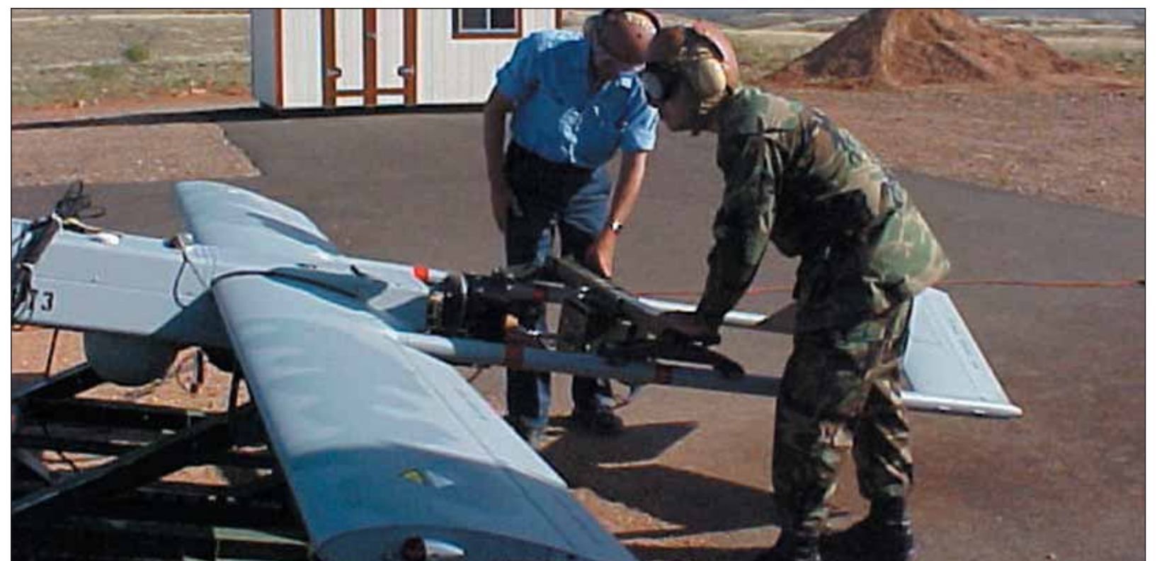
(Above) Spc. Steven N. Feeney of the Pennsylvania Army National Guard hones his skills as a new UAV pilot on the flight simulator. (Below) Sgt. Christian V. Villalva, a UAV crew chief with the Maryland Army National Guard, places a Shadow onto the launch platform to ready it for flight.
