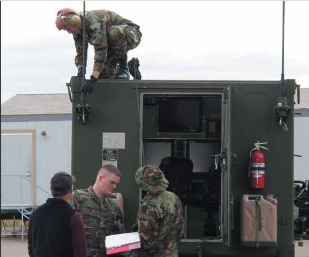
(Above) Spc. Morrongoillo of the Pennsylvania Army National Guard connects the antenna to the top of the ground control station before flight operations can begin. (Right) Sgt. Christian V. Villalva, a UAV crew chief with the Maryland Army National Guard, is handed the launch control panel during a training flight. (Below) Fly-by-wire takes on a new meaning when operating the Shadow from a keyboard.
