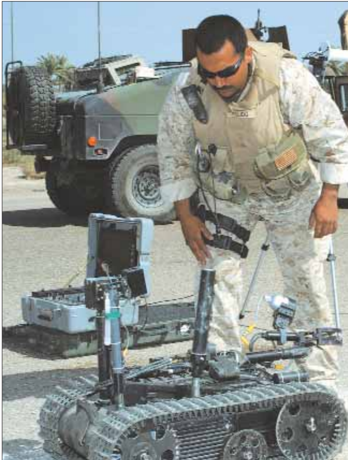
A member of the 15th Marine Expeditionary Unit assigned to Explosive Ordnance Team 8 prepares a Talon II remote-controlled robot to go down range and investigate a possible IED on the shoulder of a busy highway in southern Iraq.
