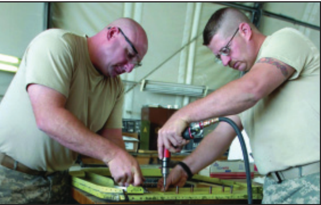
Photo by Sgt. Thomas Day Staff Sgt. Joseph Sykes (left) of the Missouri National Guard and Sgt. Gregory Harell (right) of the Mississippi National Guard work on sheet metal to be used to patch up a damaged door on a 10th Mountain Division helicopter at Bagram Air Base, Afghanistan, in October.
