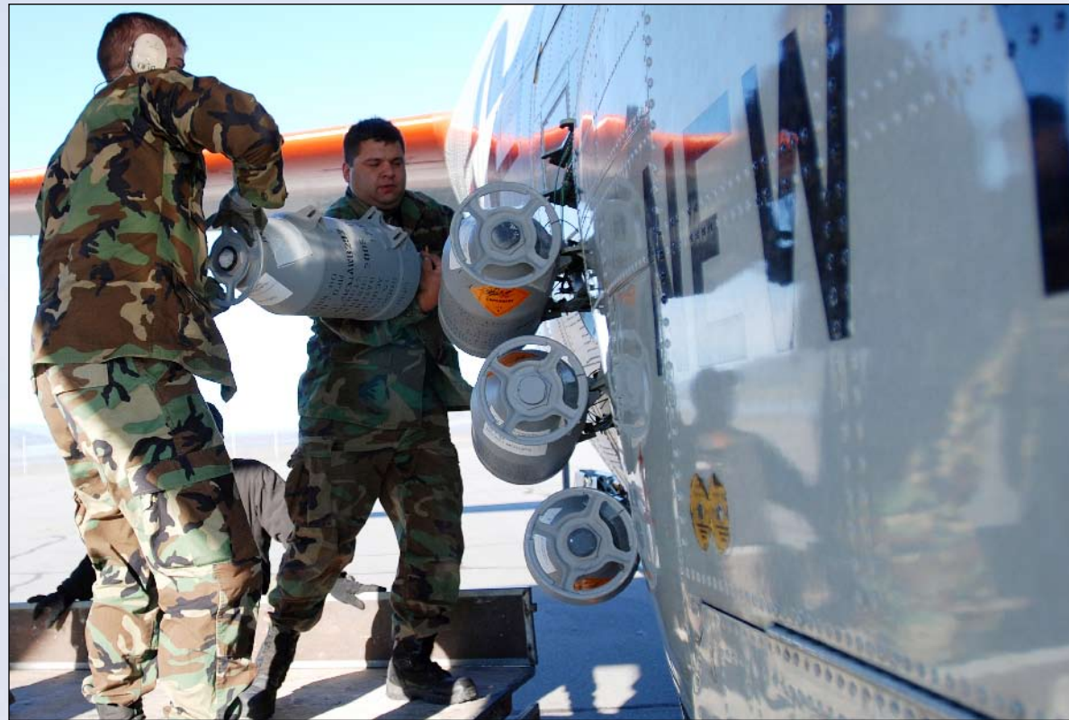
Airmen from the 109th Airlift Wing Maintenance Squadron attach Jet Assisted Takeoff (JATO) bottles to an LC-130 Hercules “skibird” on the flight line at Kangerlussuaq Airport, Greenland. A thrust of JATO provides a few extra knots of speed to pull the aircraft’s nose up from skiways on the Greenland ice sheet.
