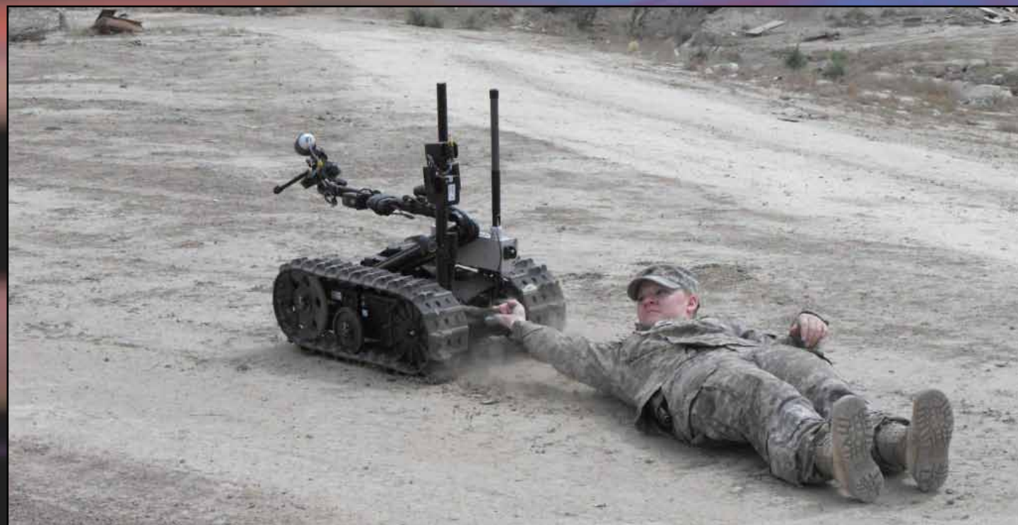
DRAGGED: While being dragged, Louisiana National Guard's 225th Engineer Brigade Soldier Sgt. Kasandra Deutsch demonstrates the power of the Talon robot, during a training exercise with the 9th Iraqi Army Engineer Regiment. The Talon robot system is used to help clear improvised explosive devices. (Photo by Maj. Pat Simon)
