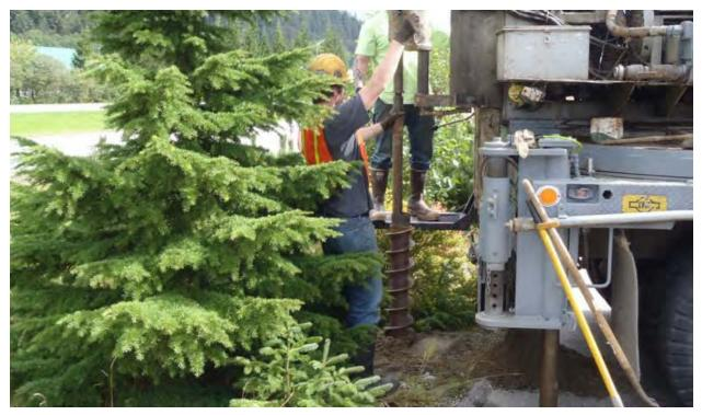
**Photo 9**: Boring B17 was located north of the paved parking area north of the hangar, and was advanced to characterize soil in the vicinity of the former oil/water separator outfall. Photo taken facing east (August 26, 2010).
