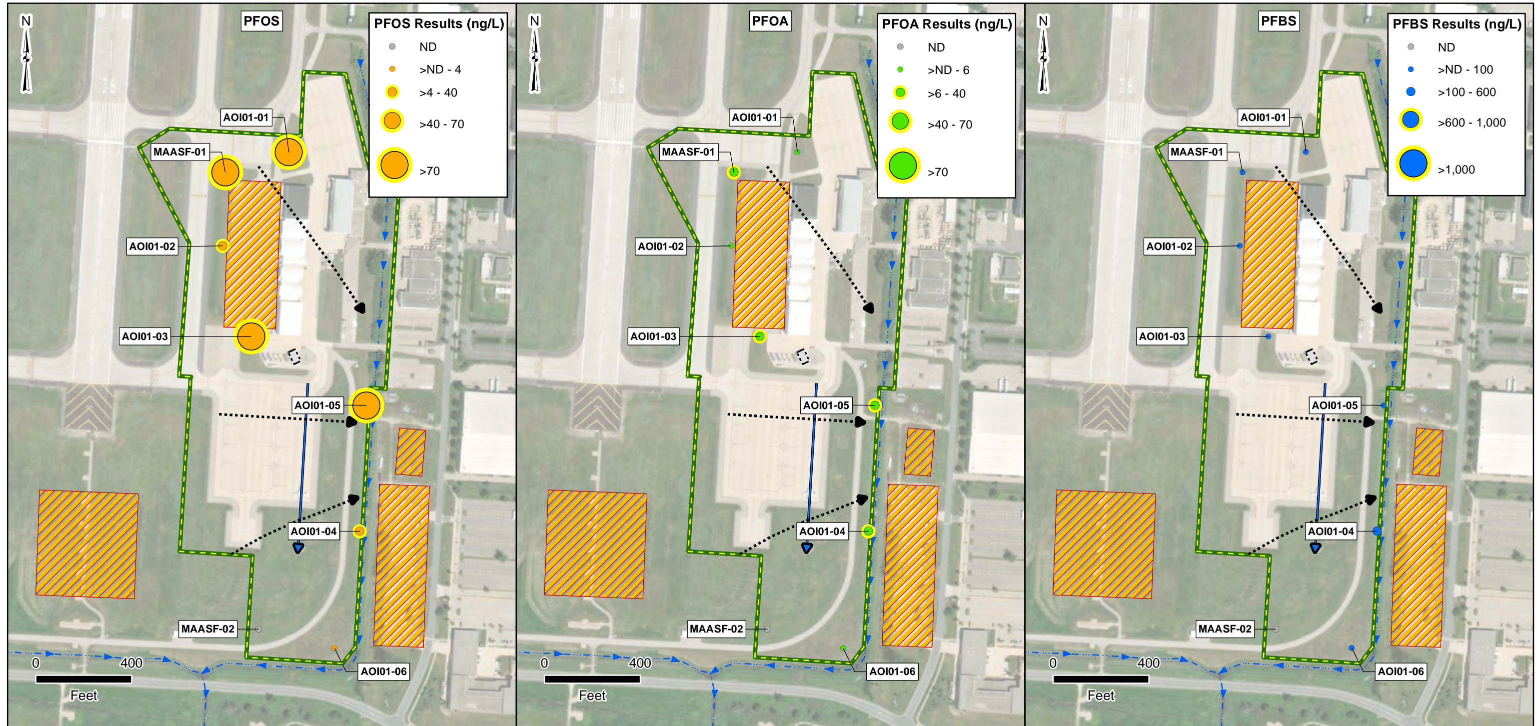
Figure 6-6 PFOS, PFOA & PFBS Detections in Groundwater
