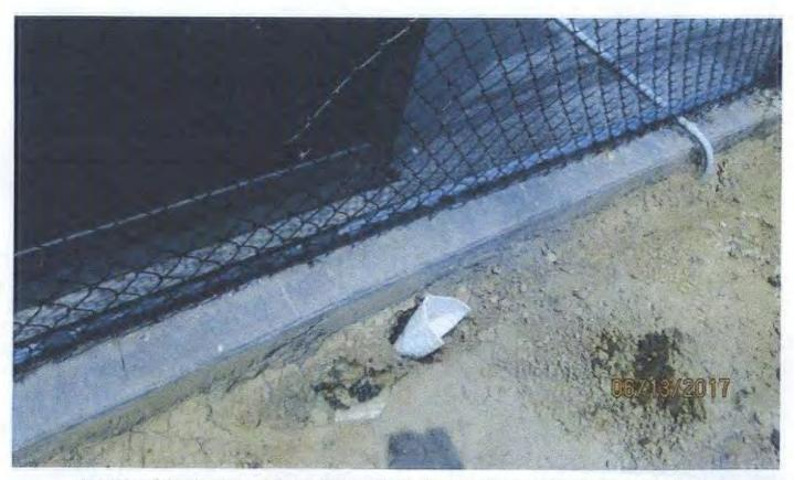
View of boring B-1 with absorbent collecting thin layer of free product observed on the surface of water within the boring.
