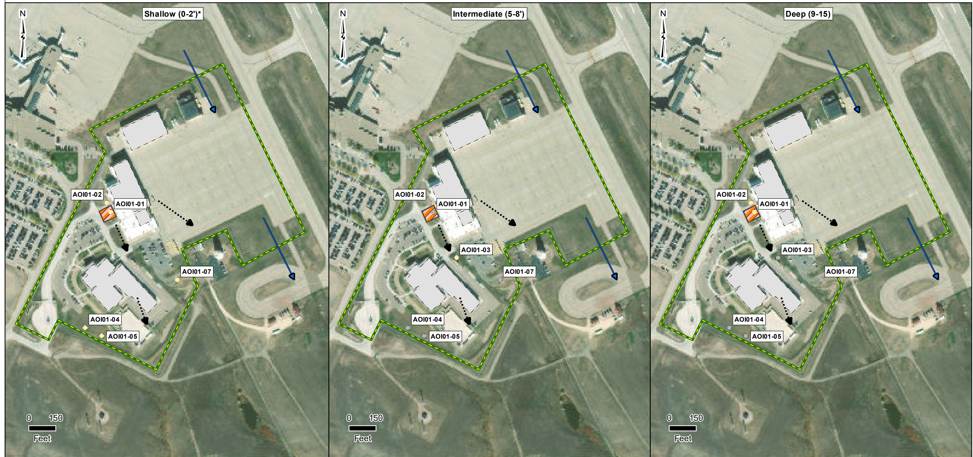
Figure 6-2 PFOS Detections in Soil
