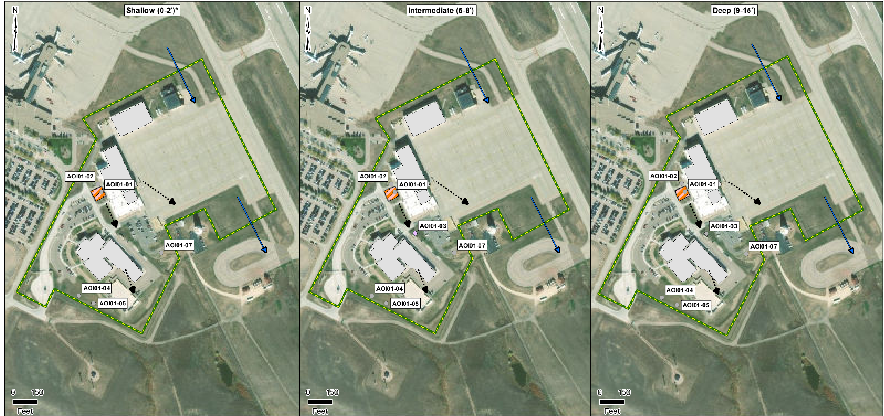
Figure 6-4 PFHxS Detections in Soil
