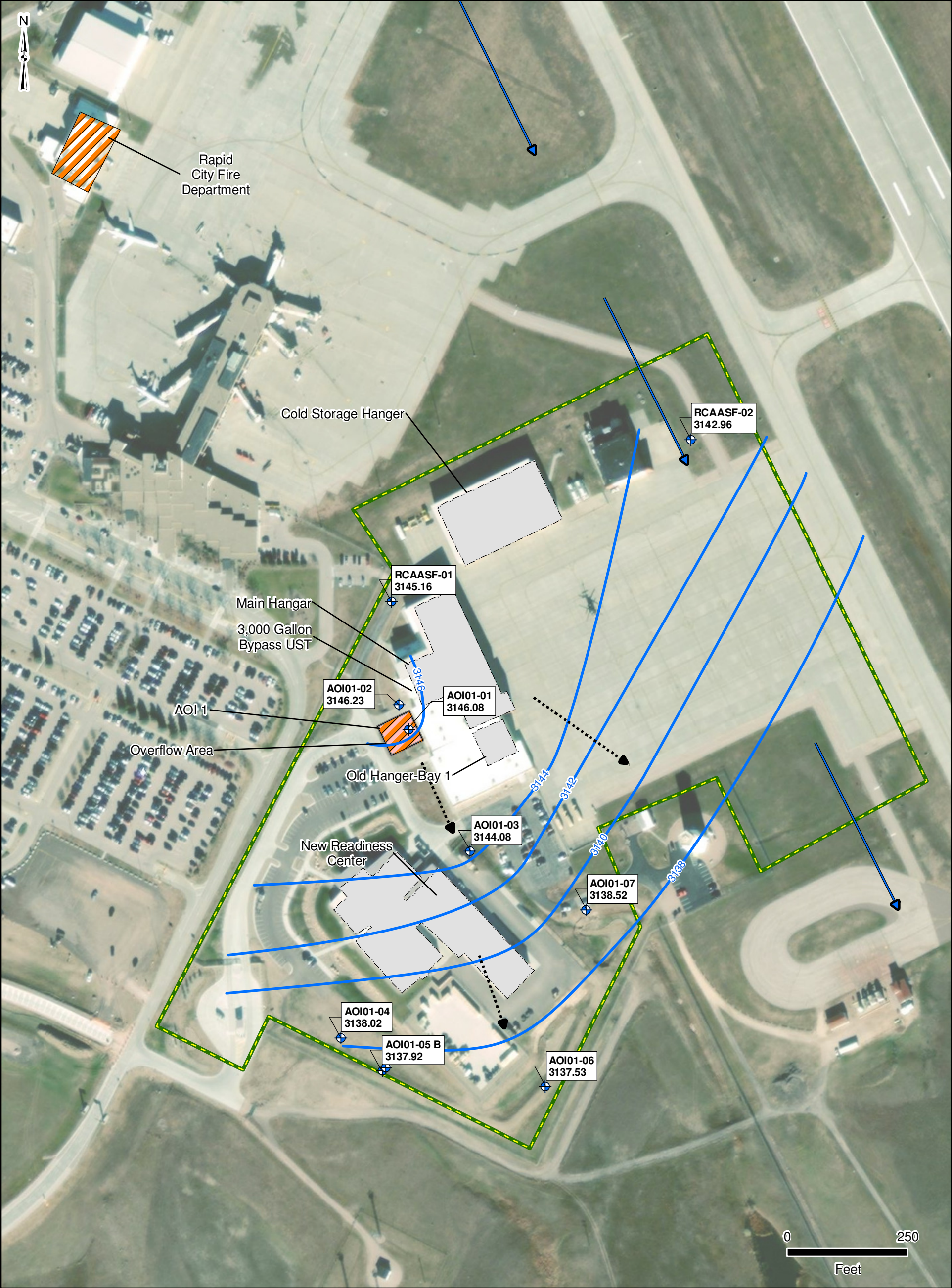
Figure 2-5 Groundwater Elevations, November 2021
