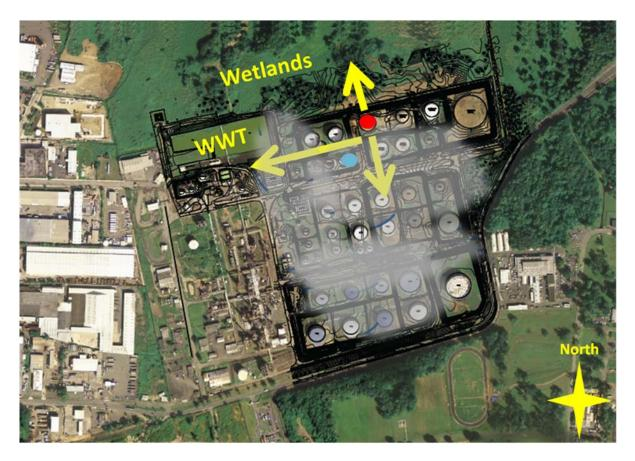
Figure 7. Topographic Survey of CAPECO Tank Farm showing the gasoline vapor cloud migration from higher elevation (Tank 409-Red and Tank 411-Blue) toward low-lying areas by the WWT plant, the south eastern end of the refinery and wetlands to the north. The cloud indicates the approximate area where the vapor cloud migrated based on surveillance footage.
