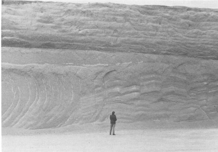
Figure 47. Working face at a pit operated by the Central Oregon Pumice Company at the Bend pumice deposit. Movable thickness of white lump pumice is about 25 feet (8 m).
