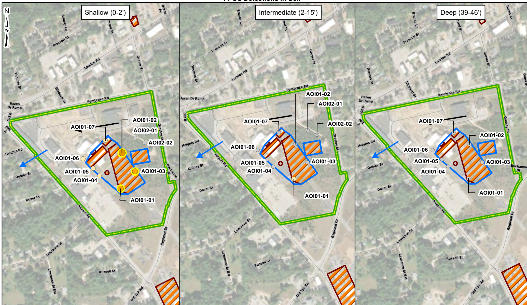
Figure 6-1 PFOS Detections in Soil
