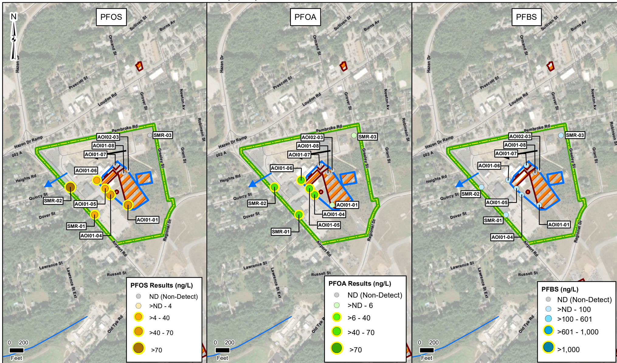
Figure 6-6 PFOS, PFOA, and PFBS Detections in Groundwater
