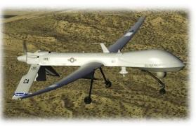
illuminator into a single sensor package. The aircraft can employ two laser-guided AGM-114 Hellfire missiles. Additionally, the MQ-1 is a theater asset for reconnaissance, surveillance and target acquisition organic to the Joint Force Air Component Commander's (JFACC) forces. The MQ-1 Predator is flown by ND, AZ, TX, OH and CA Air National Guard (ANG) units. The NV ANG supports active duty MQ-1 operational and training sorties.
