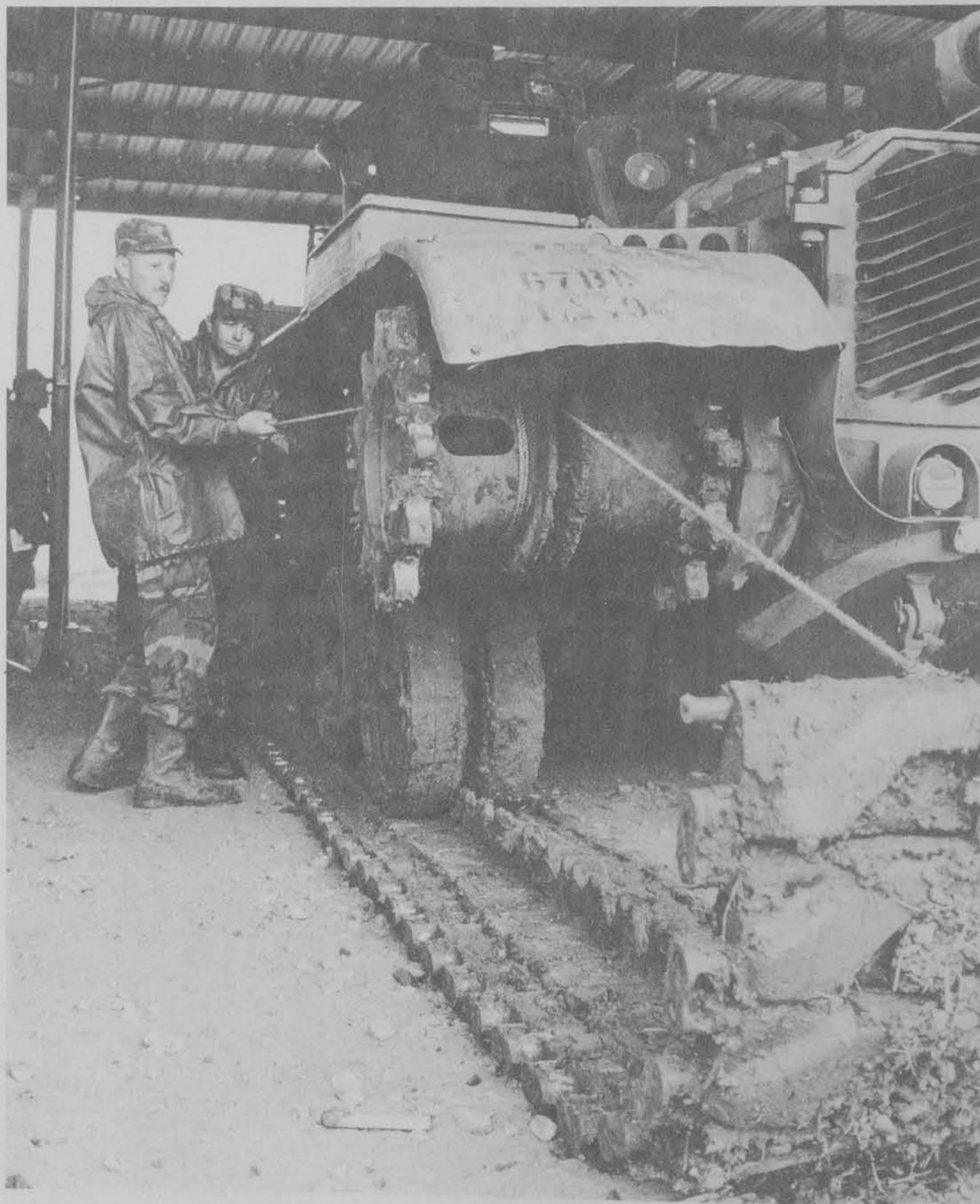
Tank crew from the 1st Bn, 195th Armor, Nebraska ARNG replaces a track.
