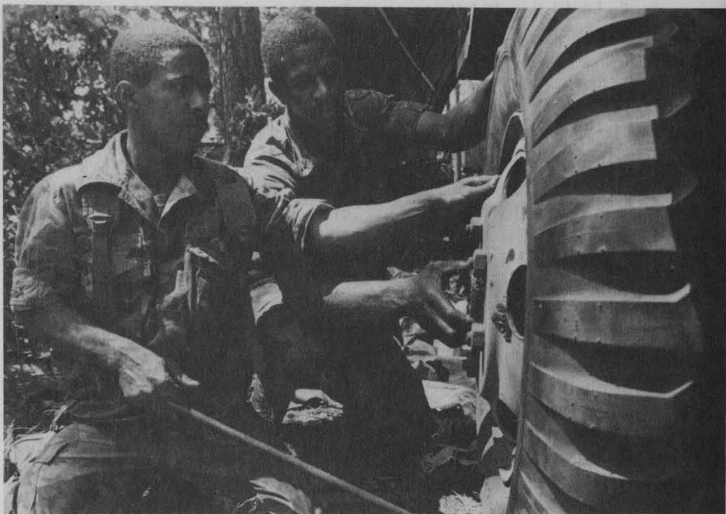
Two mechanics from Co C, 230th Spt Bn, North Carolina ARNG, change a tire.
