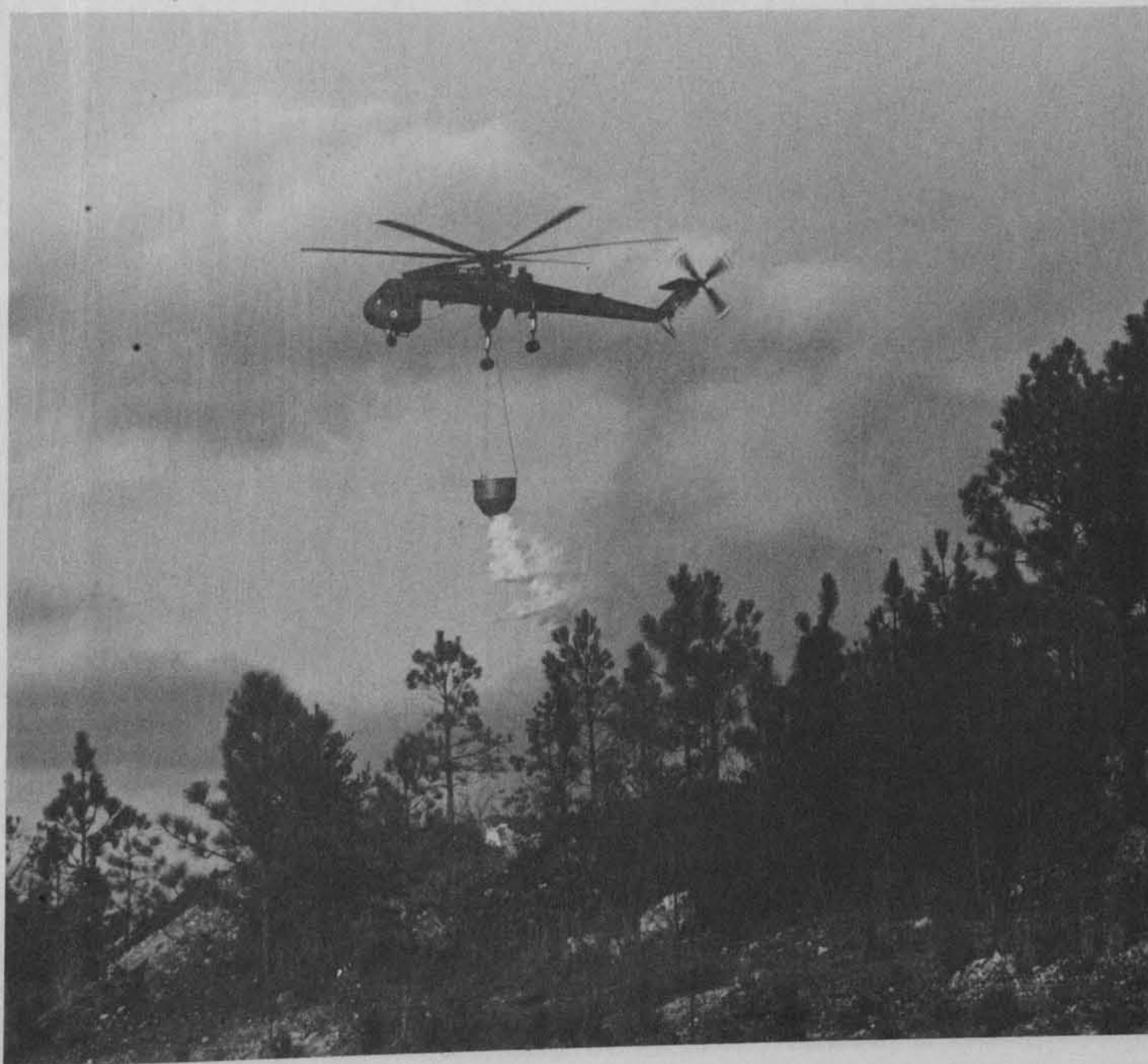
An Alabama Army Guard CH-54B "Skycrane" drops water from a 2,000 gallon water bucket to extinguish fire below. The new fire supporting effort is the result of a cooperative effort between the Alabama Guard and the State Forestry Commission to extinguish otherwise inaccessible fires in the state forests.
