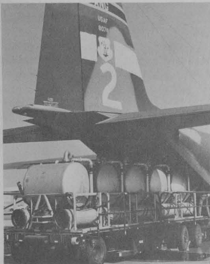
The modular Airborne Firefighting System (MAFFS) unit from the 146th Tactical Air-lift Wing, California Air National Guard takes less than 90 minutes to load and assemble in preparing for a mission.
