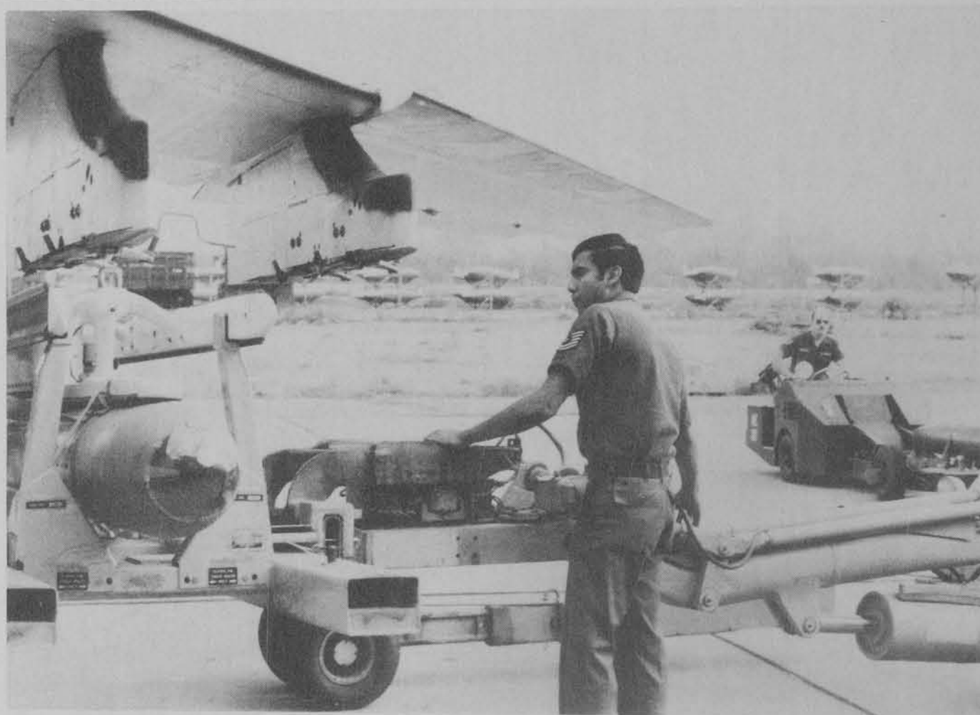
TSGT Arnaldo L. Amador, New Mexico Air National Guard, weapons technician guides a Maverick Missile into proper position for attaching to the A7D aircraft pylon.
