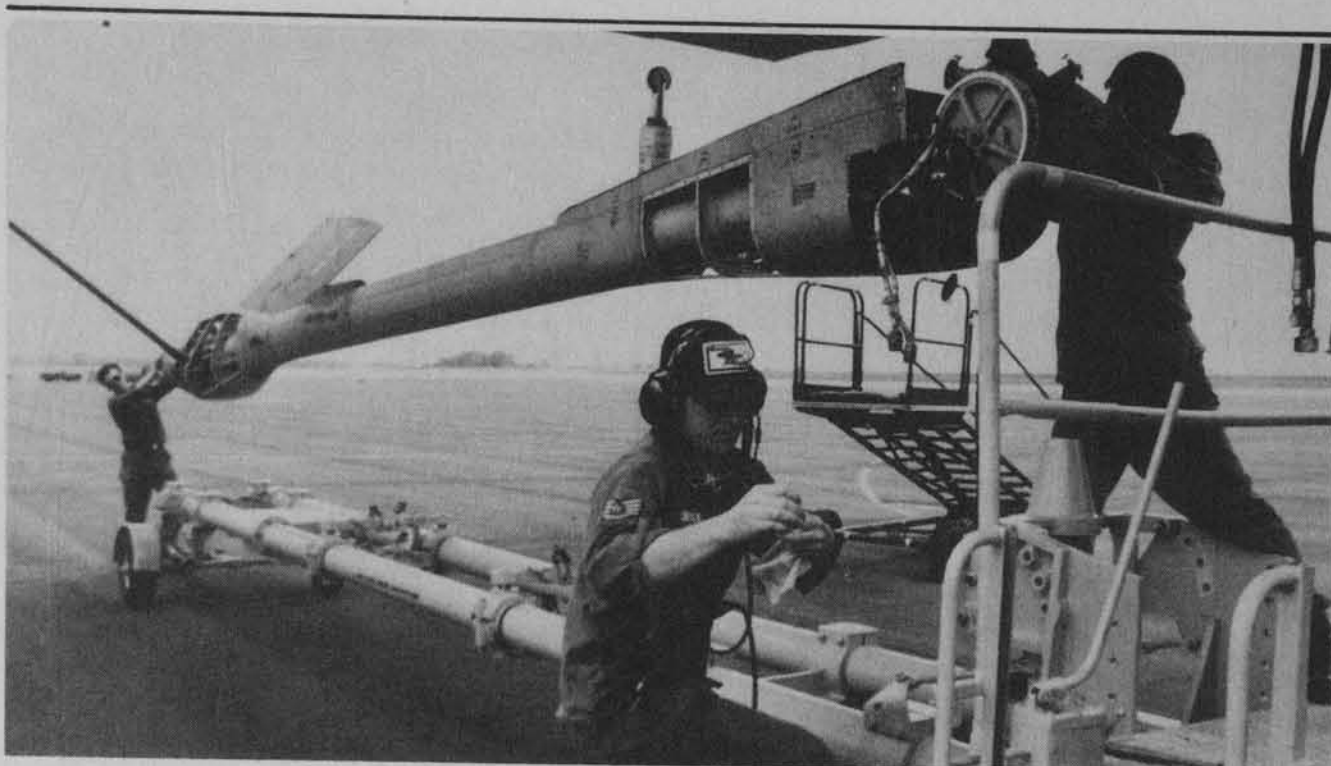
Members of the Kansas Air National Guard, 190th Air Refueling Group perform maintenance on the refueling boom of a KC-135.
