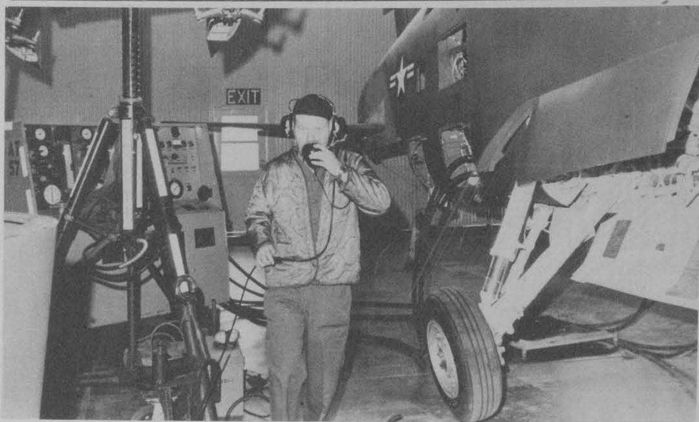
MSGT Elwood C. Acree, New Mexico Air National Guard, hydraulic technician is purging the hydraulic system of the A7D. This is done when air gets into the hydraulic system, aircraft is purged for about two hours before all air is completely removed from the hydraulic system.
