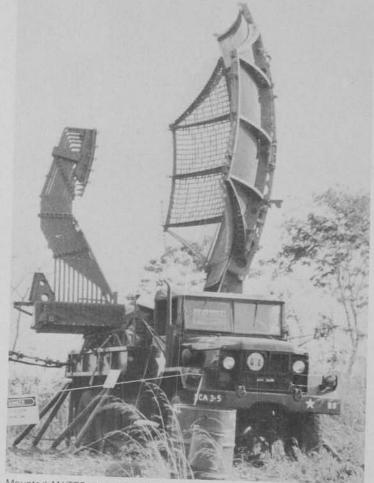
Mounted AN/TPS-43 radar set prepared for action in a field environment.
