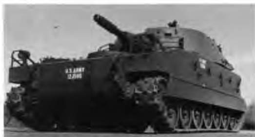
Self-Propelled 105mm Special Howitzer
